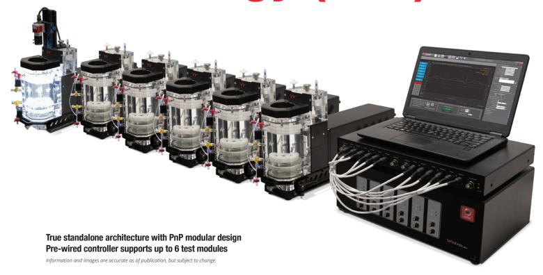
Reduce costly false negative leaflet wear results by reliably regulating test conditions during heart valve prosthesis Accelerated Wear Testing (AWT).
